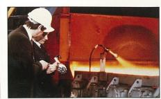
British Steel had problems removing water and scale from the surface of the hot strip. SILVENT 1212s were installed. The SILVENT products solved both a quality
