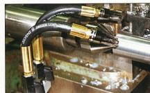
SILVENT 232, with a magnetic base, is used for blowoff in the turning of large diameter piston rods. The magnetic base fitted with flexblow hoses allows exact and easy setting of the blowing angle.
