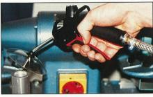
The SILVENT 007 is equipped with a unique two-step system to reduce noise levels and energy consumption. The blowing gun can easily be fitted with a transparent safety shield that protects eyes against flying debris.
