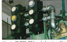
Using two ED 2033s SKF has solved a noise problem in a powder press. Connecting the silencers in series provided the expansion volume required to avoid back-pressure in the system.
