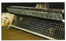
Belin, France's leading biscuit maker has installed SILVENT air knives, with twenty 920s each. The air knives blow away biscuit crumbs. The installation
