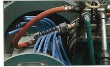
The picture shows 15 hose silencers, SDR, mounted on a 3" exhaust pipe from a pressure casting press. The risk of hearing loss has been entirely eliminated.
