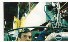
When a CD was installed at Scania, the machine was suddenly so quiet that the personnel thought there was something wrong with the machine. The noise peaks were reduced from 105 to 84 dB(A).
