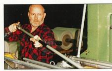
When manufacturing fabric, machine cylinders must be blown clean on a regular basis. A 753 gun fitted with a 1500 mm extension effectively reaches into the
