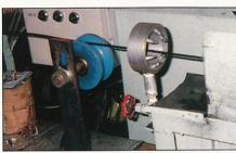
The picture shows a SILVENT 456 doughnut nozzle at a Japanese cable company. The doughnut nozzle allows cables, profiles, hoses etc to be continously fed through the nozzle.
